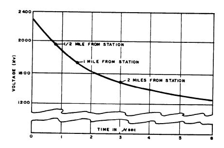
Figure 4-3. Sample power line surge voltage as a function of distance from stroke to line.
