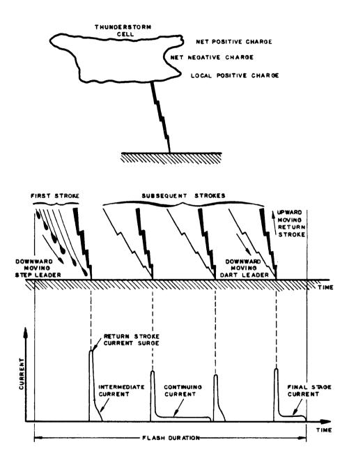
Figure 4-1. Processes and currents occurring in a flash to ground.
