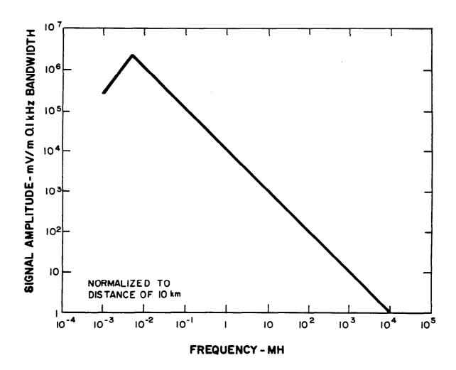
Figure 4-5. Average radiated and static fields for lightning.
