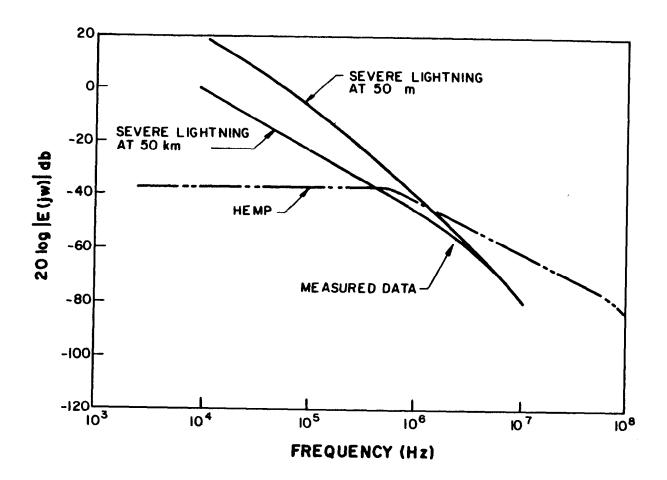
Figure 4-4. Typical spectrum of lightning radiated E-field.
