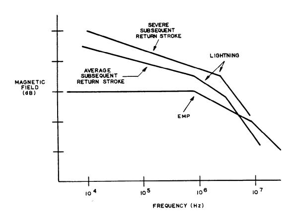
Figure 4-2. EMP and lightning comparison.
