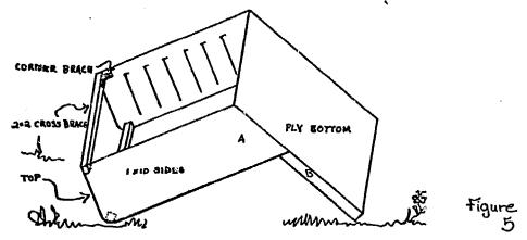
5: ASSEMBLING BODY: Turn the sides so the 1 x 4's and the curved corners touch the ground, so the sides are 4' apart. Place the 48" x 48" ply on the 1 x 4 and the 1 x 10 edges so that is is flush with the 1 x 10's (A) and overhanging the 1 x 4's by 3/4", (B).
