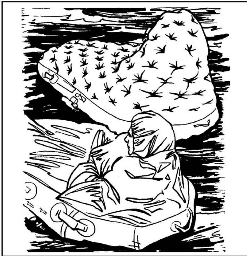
Figure 16-11. One-Man Raft With Spray Shield Inflated
