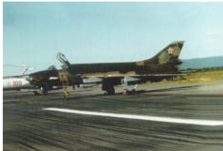
The Su-17 Fitter with its variable sweep wings, first flew in 1966. Over 1,000 were built and is in use by 19 countries. It was developed from the fixed-wing Su-7B. Export versions of this aircraft are designated Su-20 and -22. The export versions can be distinguished by a deeper dorsal spine.
