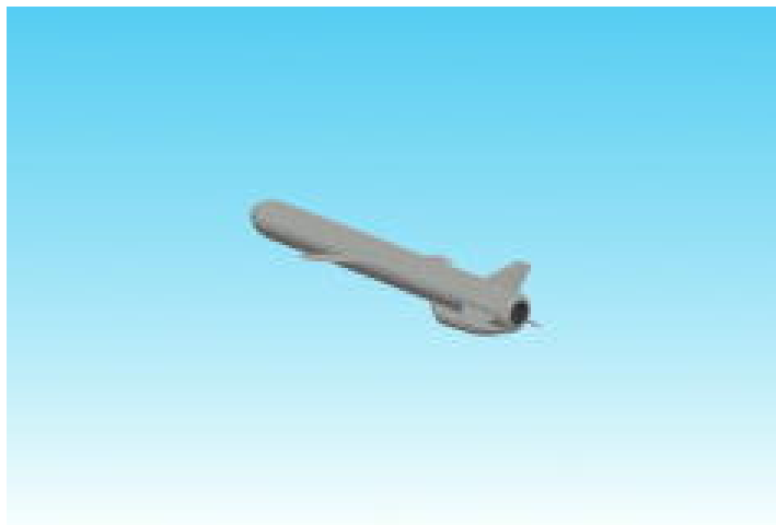
The AS-15 Kent is an intermediate-range nuclear cruise missile. The Tu-95 Bear carries 16 missiles and the Tu-160 Blackjack carries 12 missiles.
