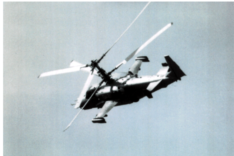
The Hokum (Werewolf), which first flew in 1982, comes with a pilots ejection seat that can be used after the main rotors have been blown away.
