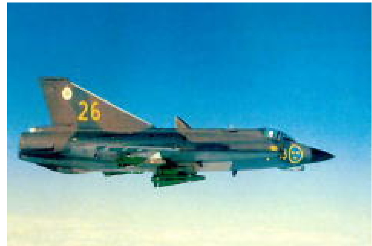
The Draken was first flown in 1955. There are several versions of this aircraft and this type can operate from small airfields. Note the unusual double-delta wing.
