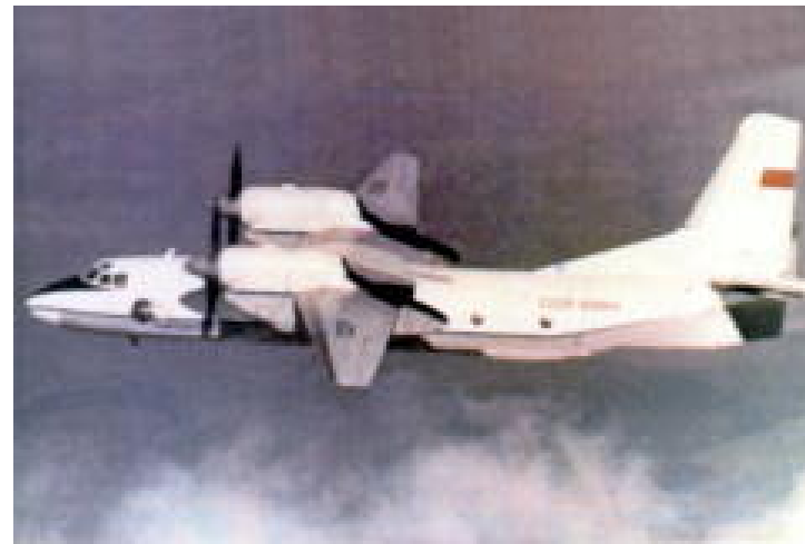
The An-32 Cline is a direct development of the An-24 Coke. Major recognition differences of the Cline are the engines mounted over the wings, and a large belly fin beneath the tail section.
