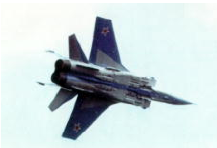
The MiG-31 Foxhound is a further development of the Foxbat, with wing and fuselage modifications. Foxhound has a look-down and shoot-down capability.
