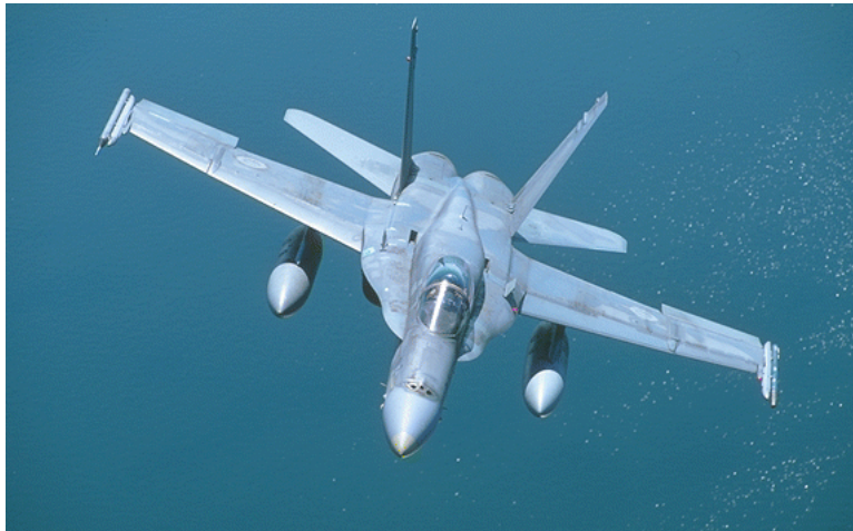
The F/A-18 Hornet first flown in 1974 and over 1,458 were built. It is used by nine countries. It is the US Navy and Marine Corps/ frontline multimission fighter. This carrier-borne and land-based attack fighter was designed to replace the aging fleet of F-4 Phantom IIs and A-7 Corsair IIs.
