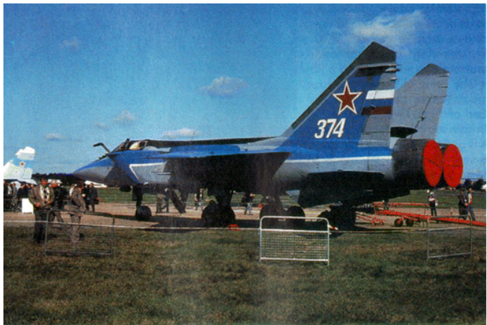
The MiG-31 Foxhound is a further development of the Foxbat, with wing and fuselage modifications. Foxhound has a look-down and shoot-down capability.
