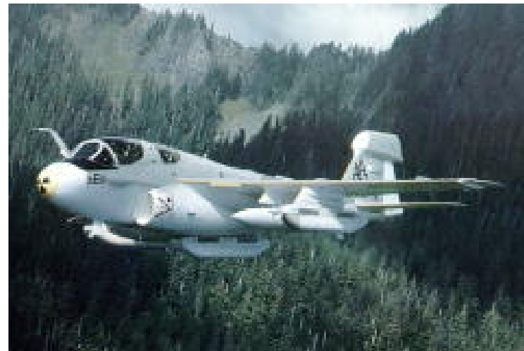
The Prowler is an advanced ECM aircraft that was used extensively in the Persian Gulf War. Another version of this aircraft was the A-6 Intruder which was used in the Viet-nam war and then retired.
