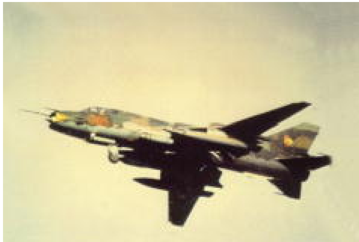
The Su-17 Fitter with its variable sweep wings, first flew in 1966. Over 1,000 were built and is in use by 19 countries. It was developed from the fixed-wing Su-7B. Export versions of this aircraft are designated Su-20 and -22. The export versions can be distinguished by a deeper dorsal spine.
