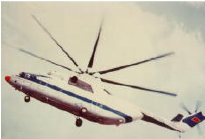
The Mi-26 Halo is the world's heaviest helicopter. It is also the first helicopter with an eight-blade rotor. First flown in 1977, the Halo became fully operational in 1983.
