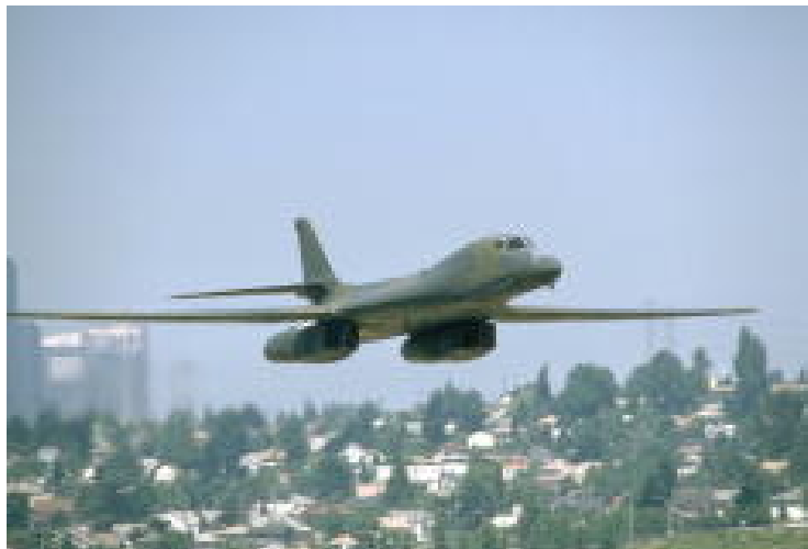
The B-1B Lancer is a long-range, low-level, supersonic, multirole, strategic bomber. The B-1B is capable of carrying conventional and nuclear weapons in large numbers.
