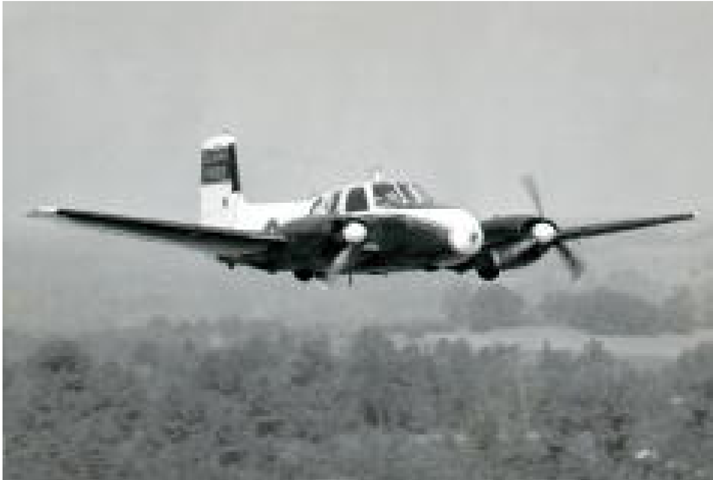
The Queen Air is in service both as an executive aircraft and a feeder liner. A model used by the US Army is the B-80, as shown here.
