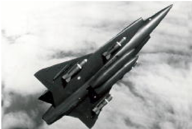
The Draken was first flown in 1955. There are several versions of this aircraft and this type can operate from small airfields. Note the unusual double-delta wing.
