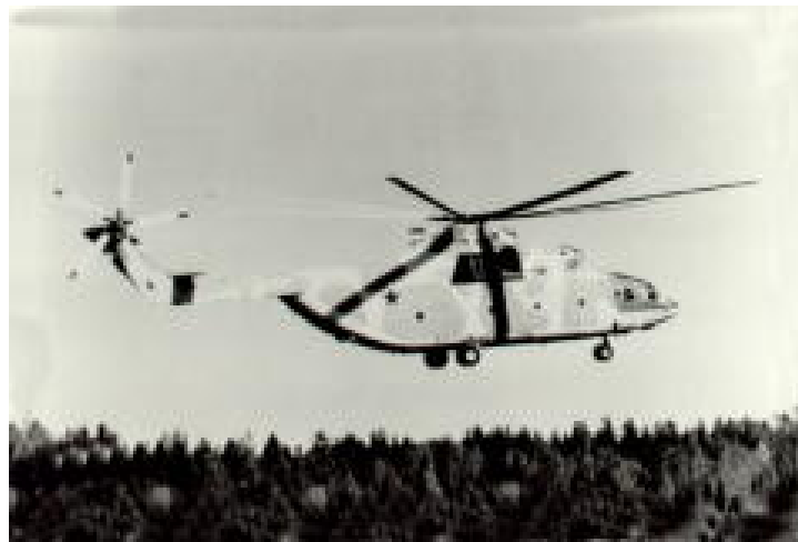
The Mi-26 Halo is the world's heaviest helicopter. It is also the first helicopter with an eight-blade rotor. First flown in 1977, the Halo became fully operational in 1983.
