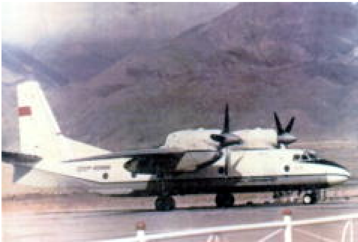
The An-32 Cline is a direct development of the An-24 Coke. Major recognition differences of the Cline are the engines mounted over the wings, and a large belly fin beneath the tail section.
