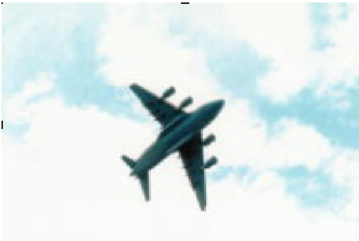
The C-17A Globemaster III is a heavy-lift cargo and troop transport plane that can accommodate three Apache helicopters with straight-in-loading.
