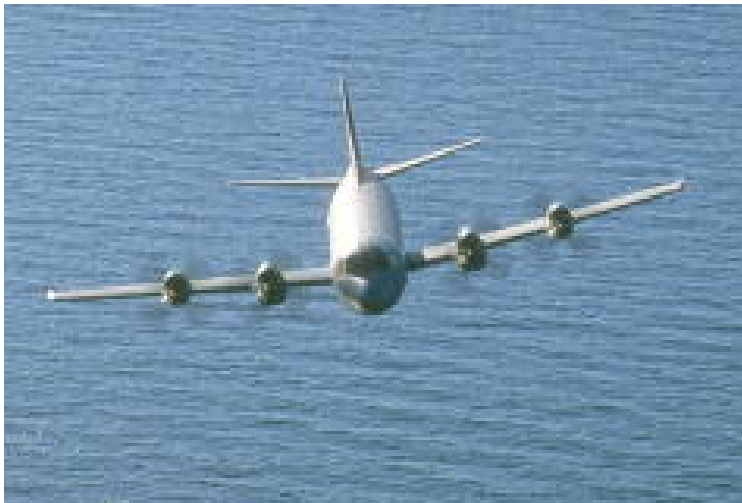
The P-3 Orion is an anti-submarine and maritime patrol aircraft which first entered service in 1962. Several versions of the P-3 have been produced and purchased by other countries making it the most widely used aircraft in the ASW field.
