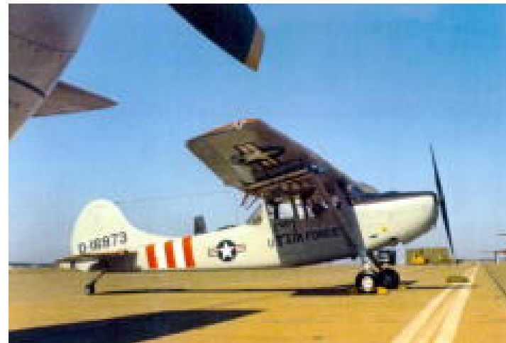
First flown in 1950, the O-1 Bird Dog was built for the US Army as a light-reconnaissance, liaison, and training aircraft. More than 3,400 were built. O-1s are in large-scale service in many countries.
