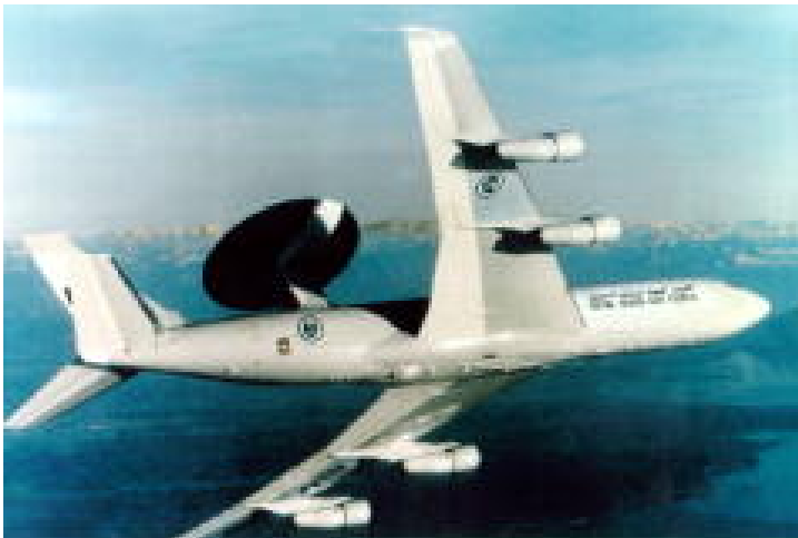
The Airborne Warning and Control System (AWACS) is an air defense operations center in the sky. The sentry's crew tracks multiple hostile targets and directs fighters to them.
