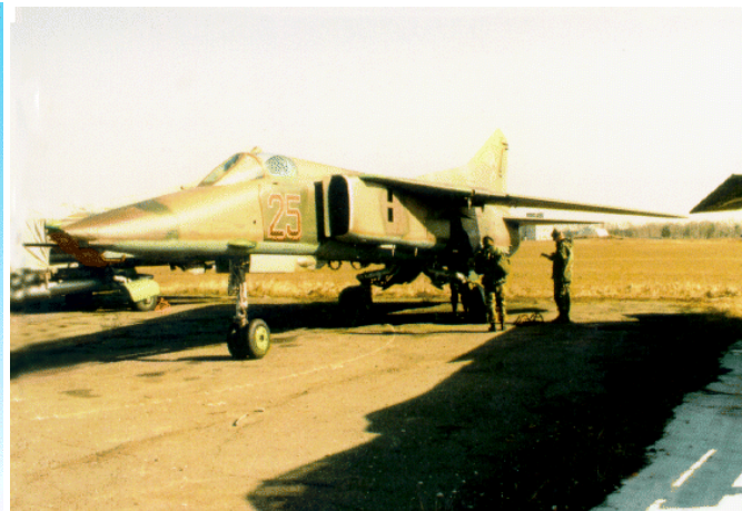
The Flogger B is a standard interceptor. The aircraft is used in Eastern Europe and the Middle East countries. Other versions of this aircraft are: C—two seater; G—improved interceptor; and E—export.
