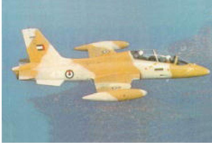
The M.B. 339A, a two-seat aircraft, was first flown in 1976. 183 of them are being used by six countries. Another version, the M.B. 339K, is a single-seat aircraft.
