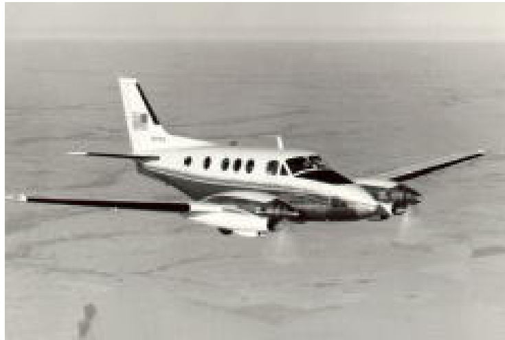
The King Air is based on the Queen Air, but with a pressurized fuselage. There are several models; the USAF advanced trainer is the T-44. More than 1,400 King Airs have been built and are in use in many countries.
