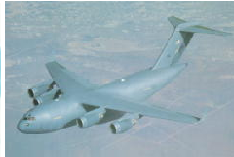
The C-17A Globemaster III is a heavy-lift cargo and troop transport plane that can accommodate three Apache helicopters with straight-in-loading.
